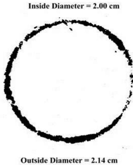
Figure 3. Print of the surface contact area of a vial
